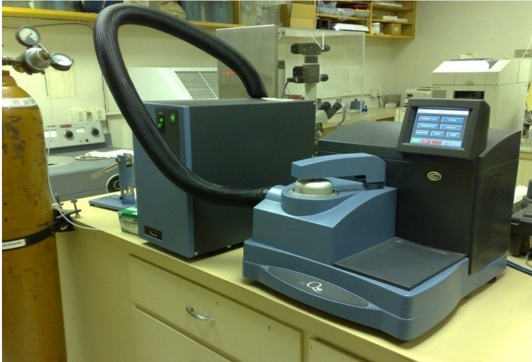
Figure 3-1. TA Instruments heat flux DSC Q100 equipped with modulated DSC connected to a refrigerated cooling system, RCS (Al-Qatami, 2011).
