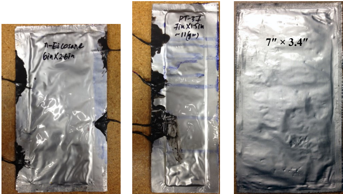
Figure 4-16 Actual photographs of PCM encapsulations: size 1 (Left), size 2 (middle), size 3 (right).
