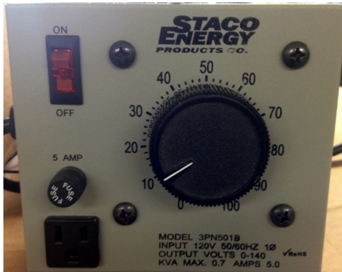
Figure 4-10 An analog variac to provide different voltages to the heater.
