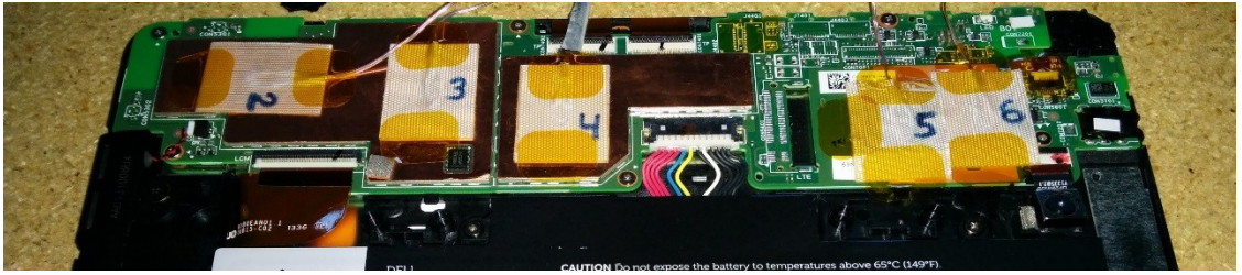
Figure A-6 Position of the five thermocouples attached on the back-side PCB of Dell Tablet PC for thermal analysis.
