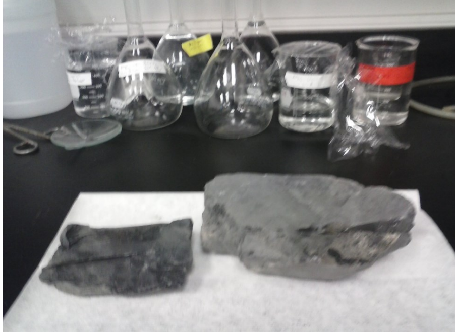
Figure 4.9.1: Samples of Meguma Slate from a construction site in down town Halifax (Queens Street, between 1358-1478)
