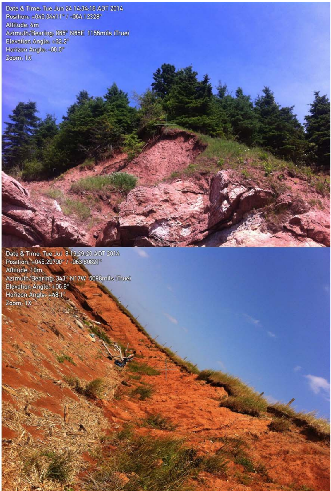
Figure 2.5: Example photographs taken with the theodolite application. Top photo shows elevation angle to top of cliff taken from 15 m out from the cliff base. Bottom photo shows the slope angle of the cliff face being measured.
