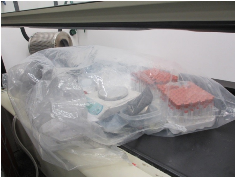
Figure 4-12 Glove bag for nano Ti sample preparation. 78
