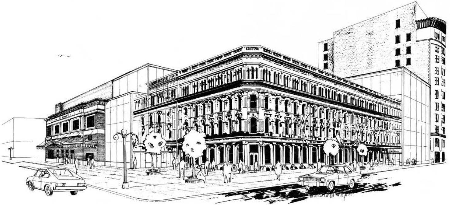
The pressed metal panels of the Empire Hotel (1884) which were put into storage following the demolition of that building are used as a facade for an addition to the Pantages Theatre, in this design proposal by the author.
