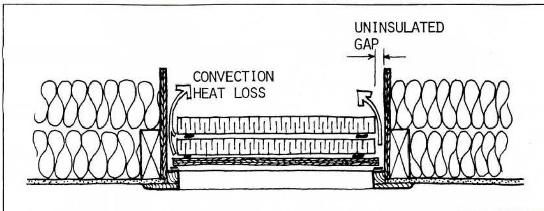
Figure 8. Typical insulated attic access hatch.
