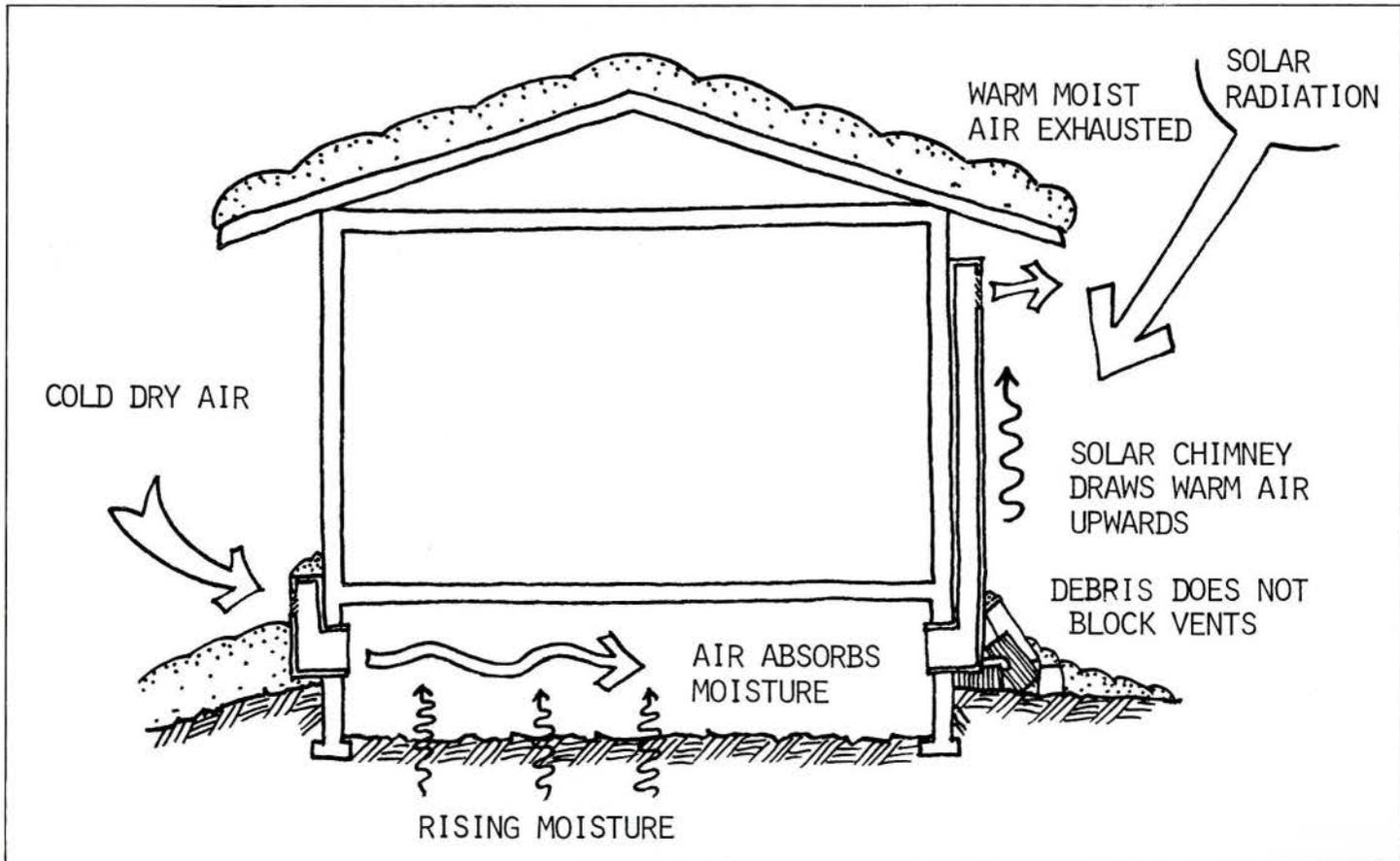
Figure 7. Proposed crawl space venting using a solar chimney.
