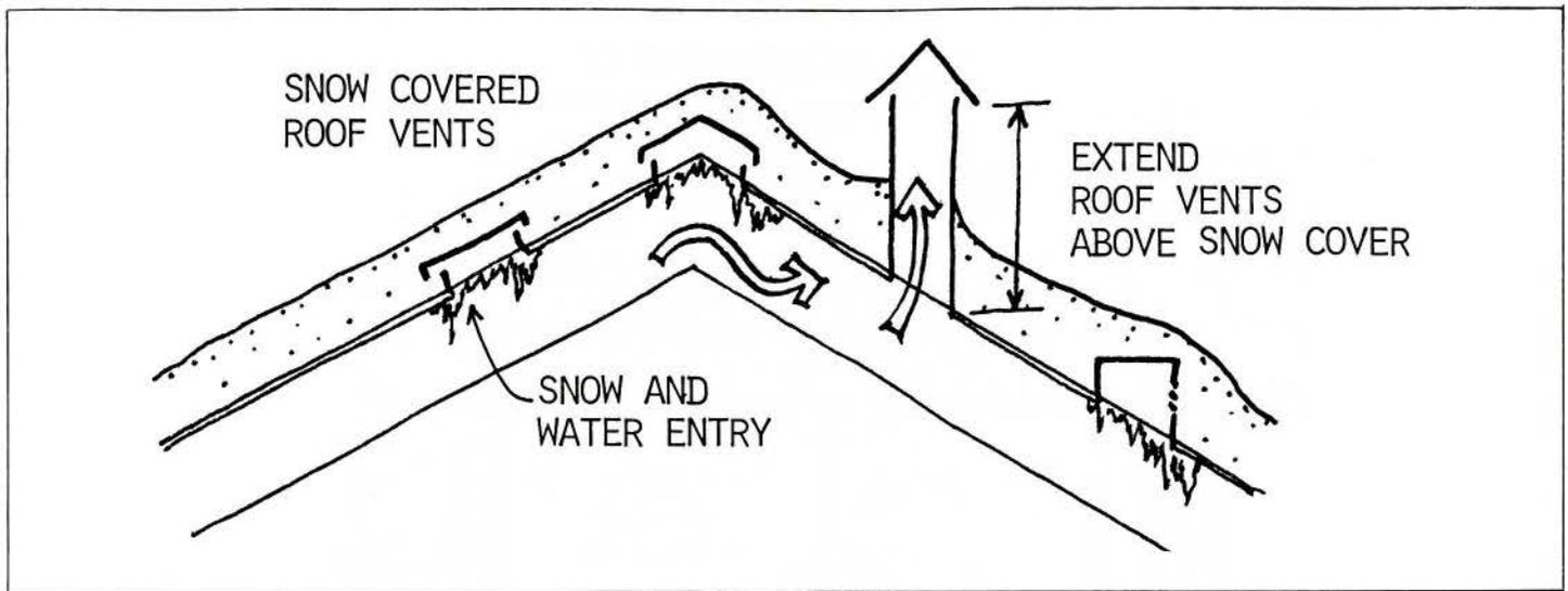
Figure 1. Attic vents must be higher than expected snow cover.
