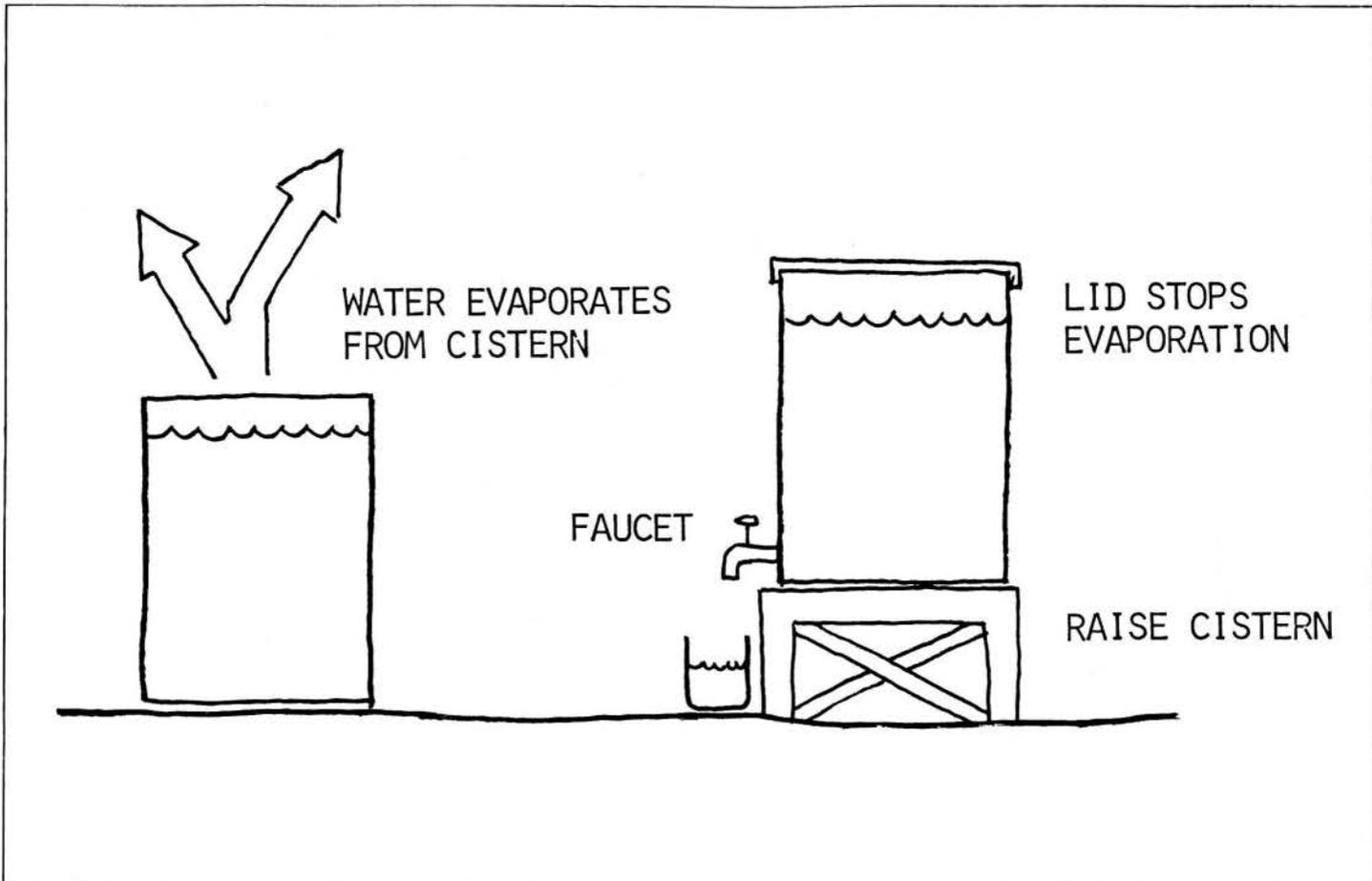
Figure 6. Water cistern for houses without plumbing.
