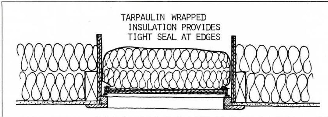
Figure 9. Proposed attic access hatch with good insulation and air seal.
