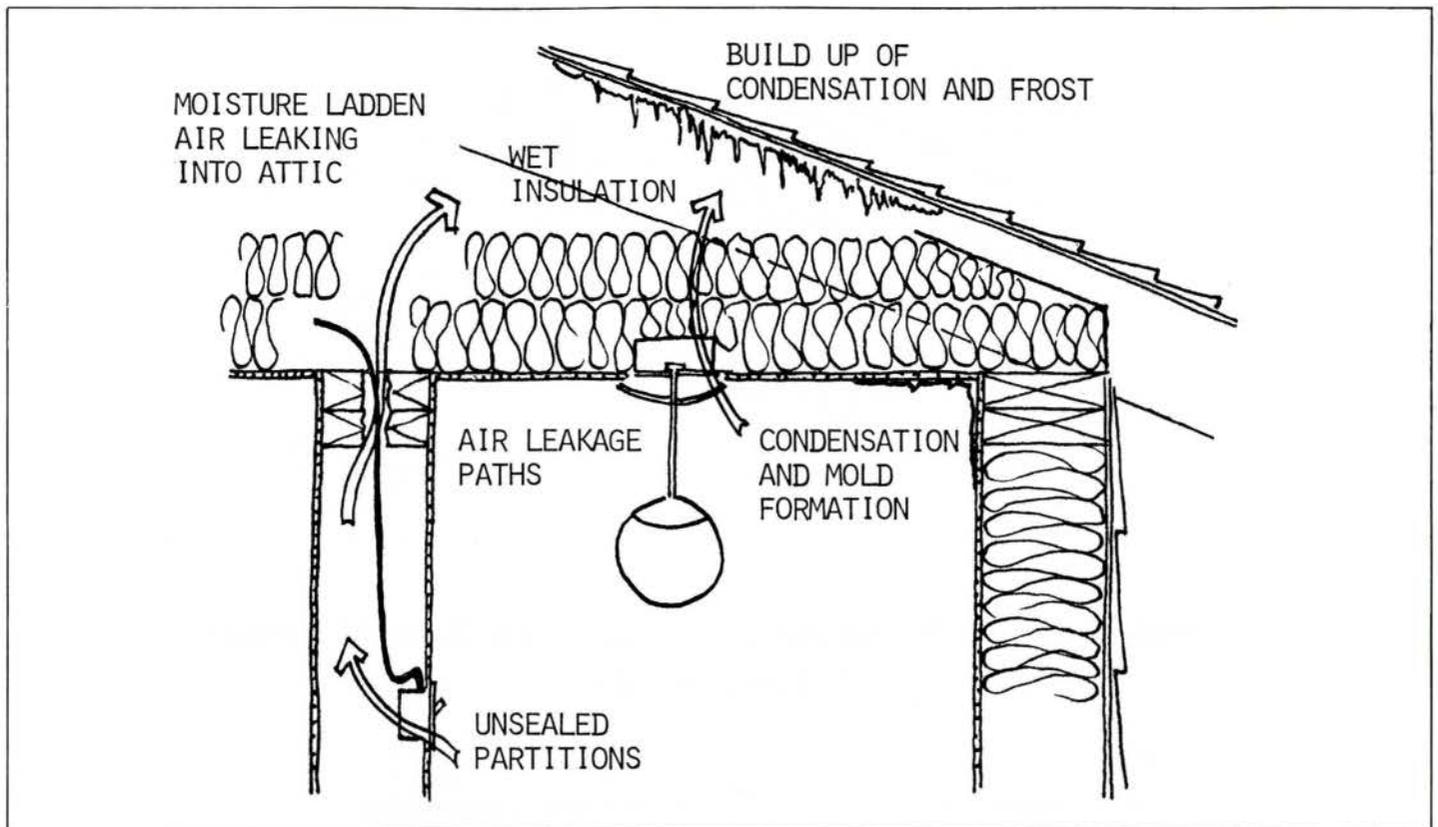
Figure 2. Attic condensation resulting from air leakage through the ceiling.
