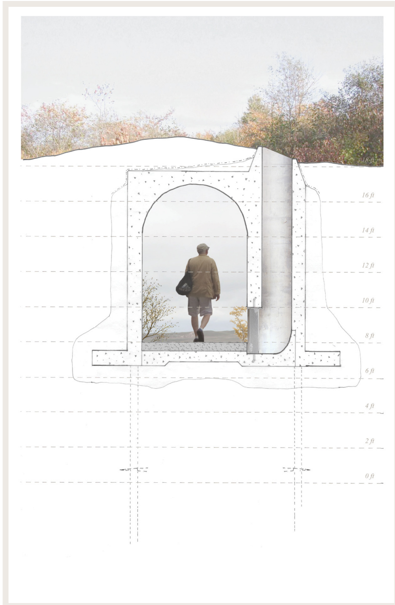
Section 5: This section is cut through the tunnel at Lower Landing. A light well brings light to the bottom of the space to create a sense of inversion.
