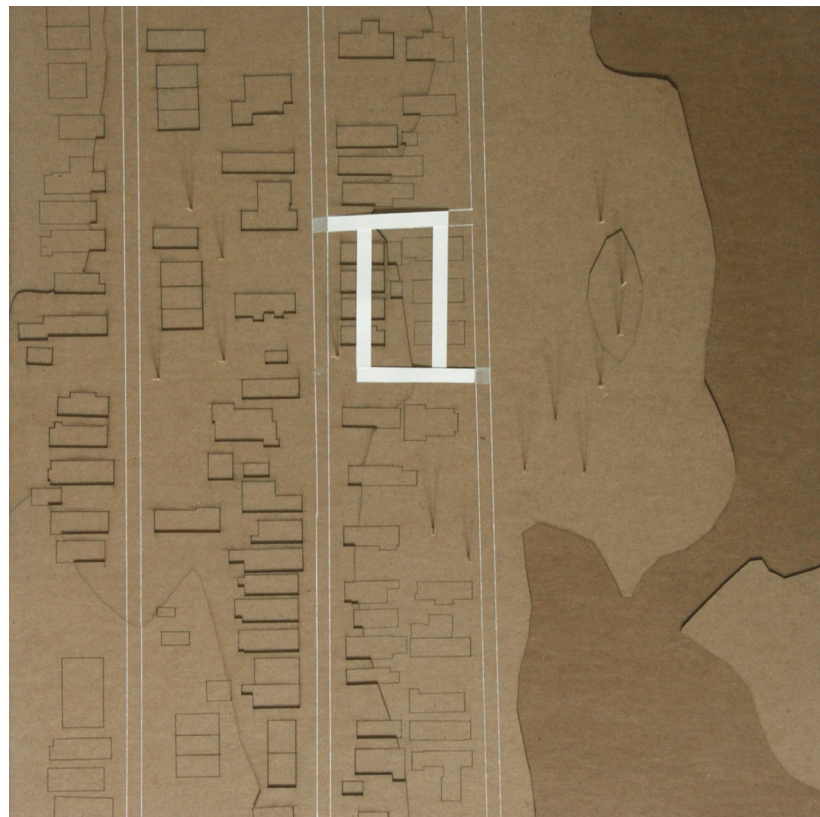
Lost Lane Loop in plan. Original model measured 17.5" by 17.5" at a scale of 1:500. Each contoured layer represents an elevation change of 2 feet.
