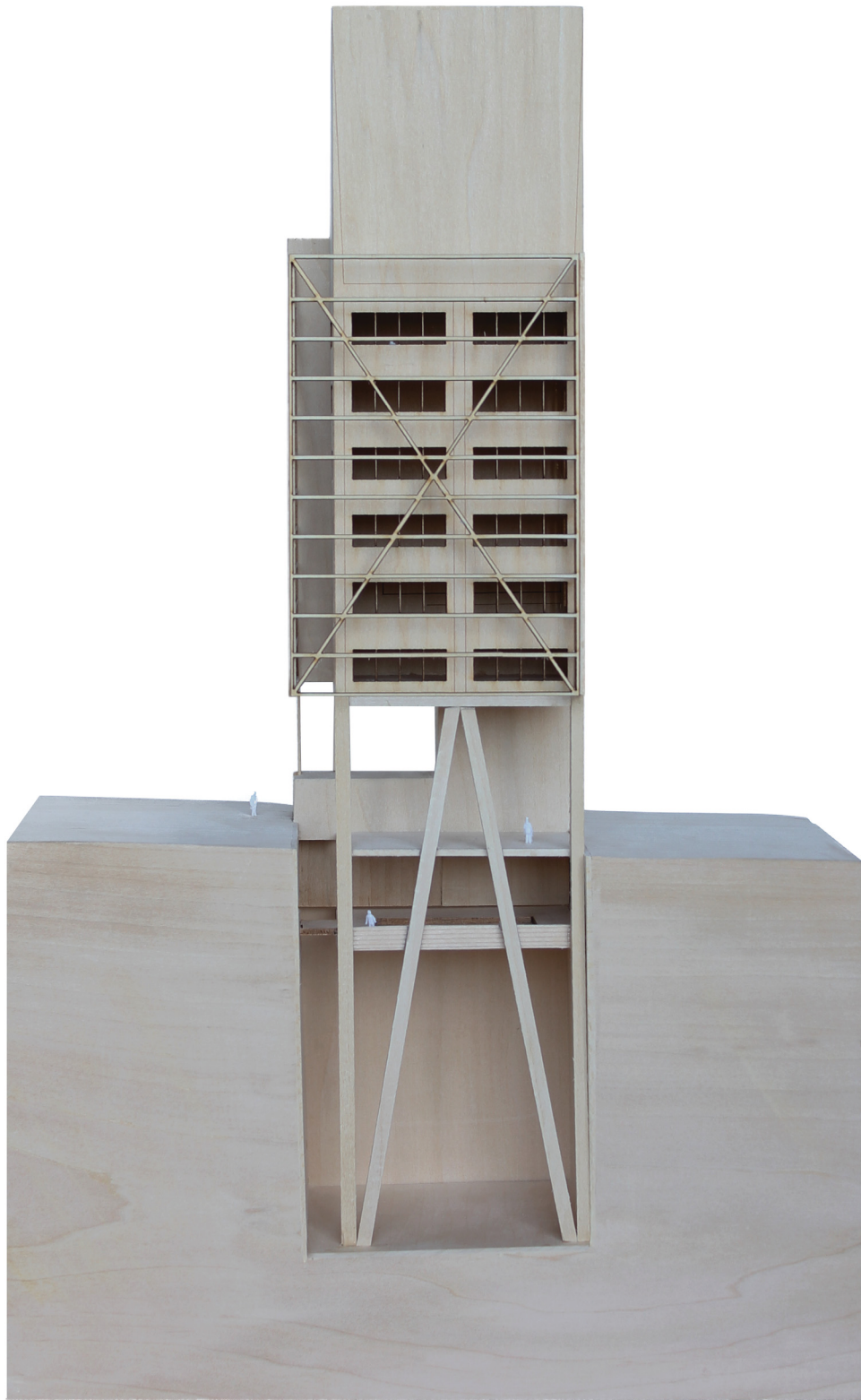
Sectional model photo. Material Basswood, model Scale 1:200. Photo not to scale.
