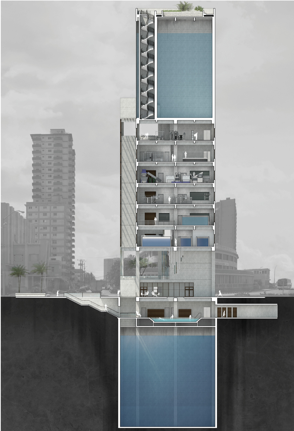
Main North-South section through building showing raw storage and filtered storage above.
