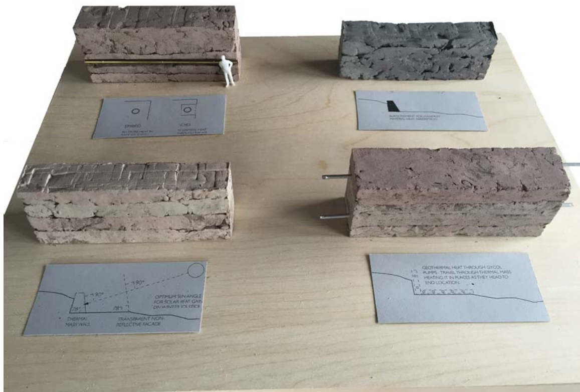
Stereotomic elements material tests. Stereotomic elements make up the retaining wall/path cutting into the slope between the buildings and the inset retaining walls hugging both buildings.
