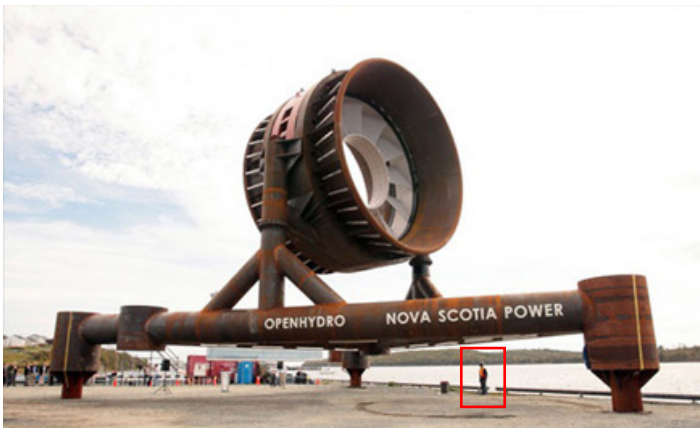
Nova Scotia Power's Open Hydro In-Stream turbine before installation in 2012. A person is highlighted under the turbine for scale.
