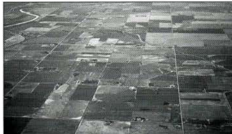
FIG. 32. ORTHOGONAL SYSTEM OF LAND DIVISION ON THE PRAIRIES. AIR VIEW. | RON WILLIAMS
