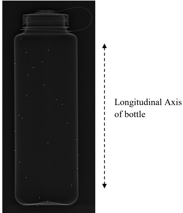
Figure 12: Radiographic representation of the calibration object used in the EOS calibration protocol.
