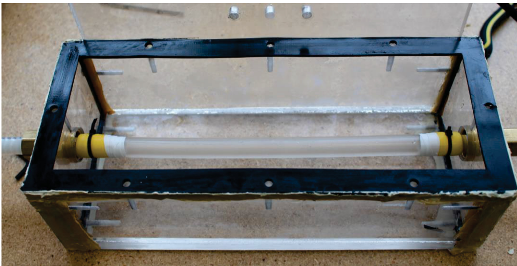
Figure 3-7 - Sylgard vessel affixed in acrylic test section
