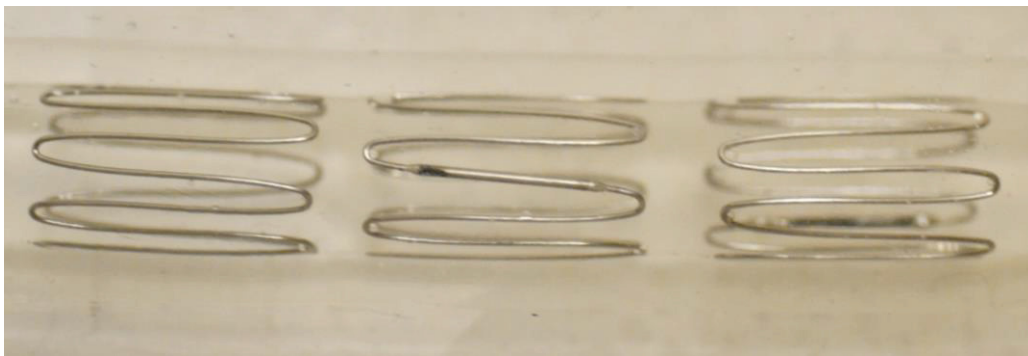
Figure 3-3 – Three 12 mm stent wires removed from their polyester cover and deployed inside a 10 mm inner diameter compliant mock artery.
