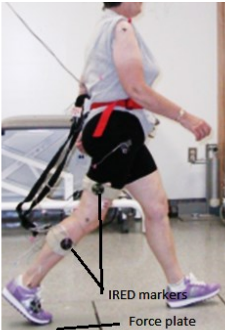
Figure 3.3: Participant walking on the force plate with the 16 IRED markers attached on the right leg.
