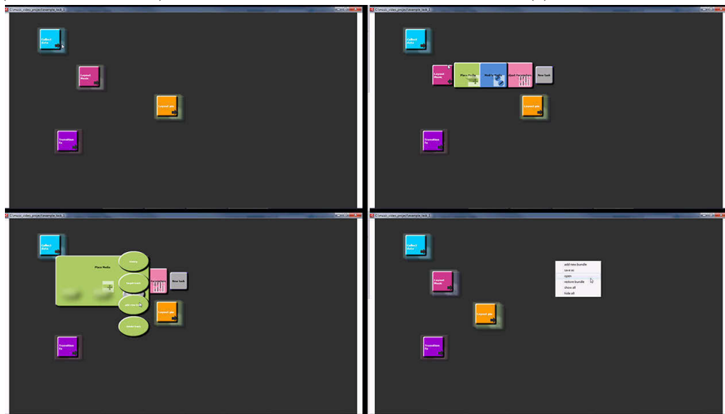
(b) A low-fidelity prototype for the early design concept. The task-view initially displays a number of objects representing action groups (top-left figure). When the user interacts with them, they reveal their child objects displaying the hierarchical structure of the task.
