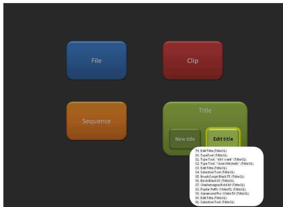
Figure 4.15: View D: a contextual view based on the menu structures. In this view, actions are grouped based on the menu grouping used in a standard MMA system (e.g., File, Clip, etc). Each menu group contains sub-menus creating a 3-level hierarchical structure.
