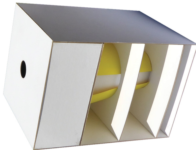
Model of middle segment of the tunnel.
