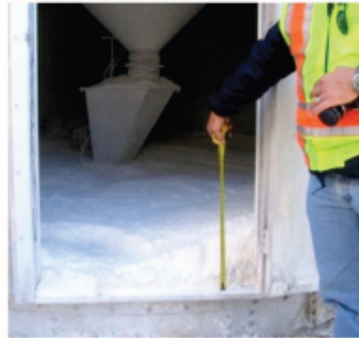
Cornstarch accumulation under cornstarch silo
