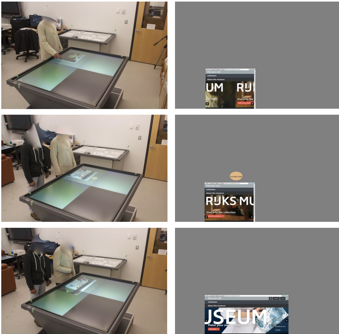
Figure 16: One user using ProximityTable (top), a new user reach the table within the intimate space of the existing user; the system recognize the new user as onlooker and notifies existing user (middle), the existing user chose to increase the size of the workspace (bottom)
