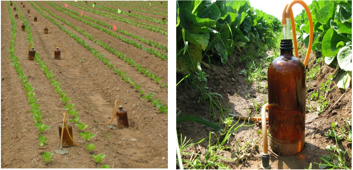
Figure 3.3. Lysimeter placement in the field
