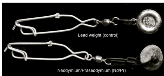
Figure 6.2: Nd/Pr alloy and lead attached to a small tuna clip using a cable tie (total length, approximately 17.5 cm). The diameters of the Nd/Pr and lead weights were approximately 3 cm.
