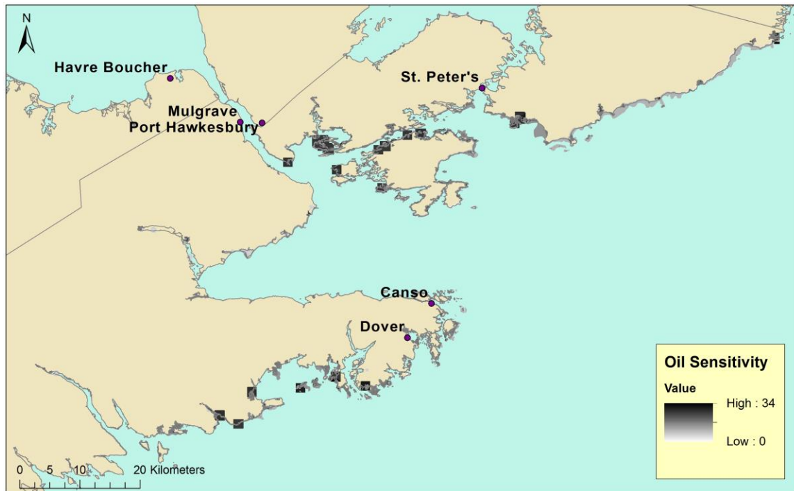
Figure 3-6. Relative sensitivity of coastal habitats to oil throughout the study site as determined by raster overlay analysis. Black squares indicate locations where sensitivity values fall within the top 25 percent of values.
