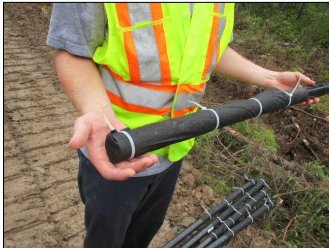
Figure 7. Shallow well with landscaping fabric covering
