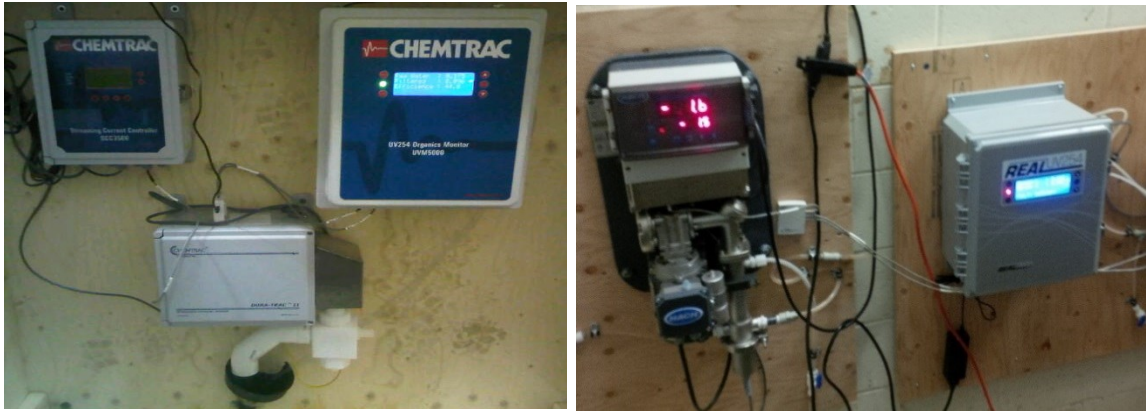
Figure 3.5: a) Chemtrac UV 254 and SCM monitors; b) RealTech UV 254 and HACH SCM monitors
