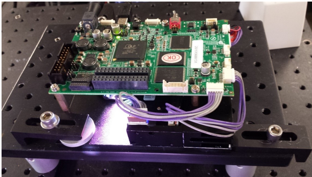
Figure 4.17: LightCrafter 4500 with its integrated optics removed. The DMD was then placed in front of the aperture at a distance equal to the focal length
