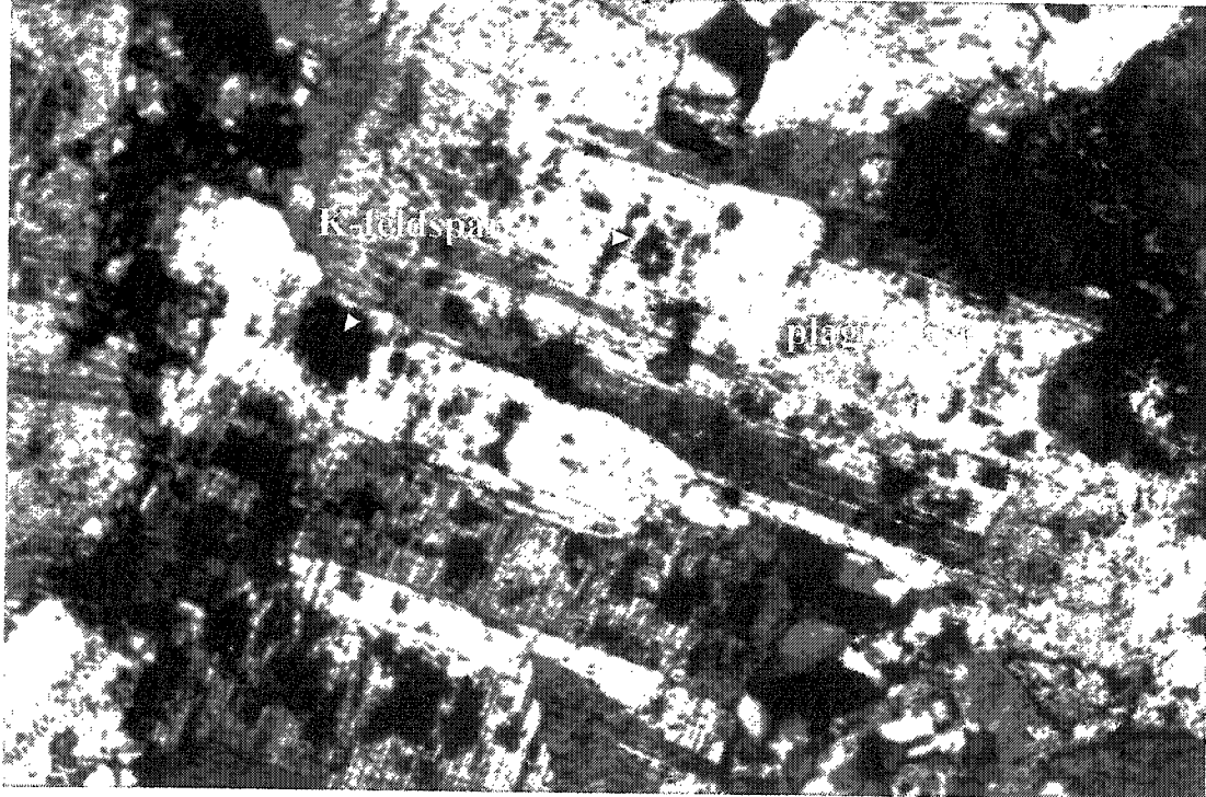
Figure 5.5. Antiperthite in the potassic alteration zone. Irregular blebs of K-feldspar occur throughout the large plagioclase grains.
