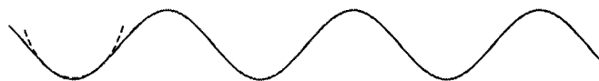
Figure 1.2: Surface potential along the surface (solid line) and its parabolic fit (dashed)
