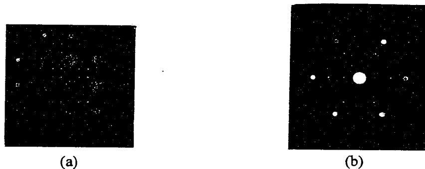
Figure 4.26 DPs recorded near (a) \langle 100 \rangle and (b) \langle 111 \rangle -types of zone axes for a Ag modified ternary alloy sample sintered 4h.
