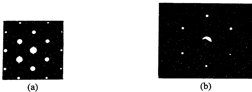
Figure 4.23 DPs recorded near (a) \langle 110 \rangle and (b) \langle 111 \rangle -types of zone axes for a ternary alloy standard sample sintered 4h.
