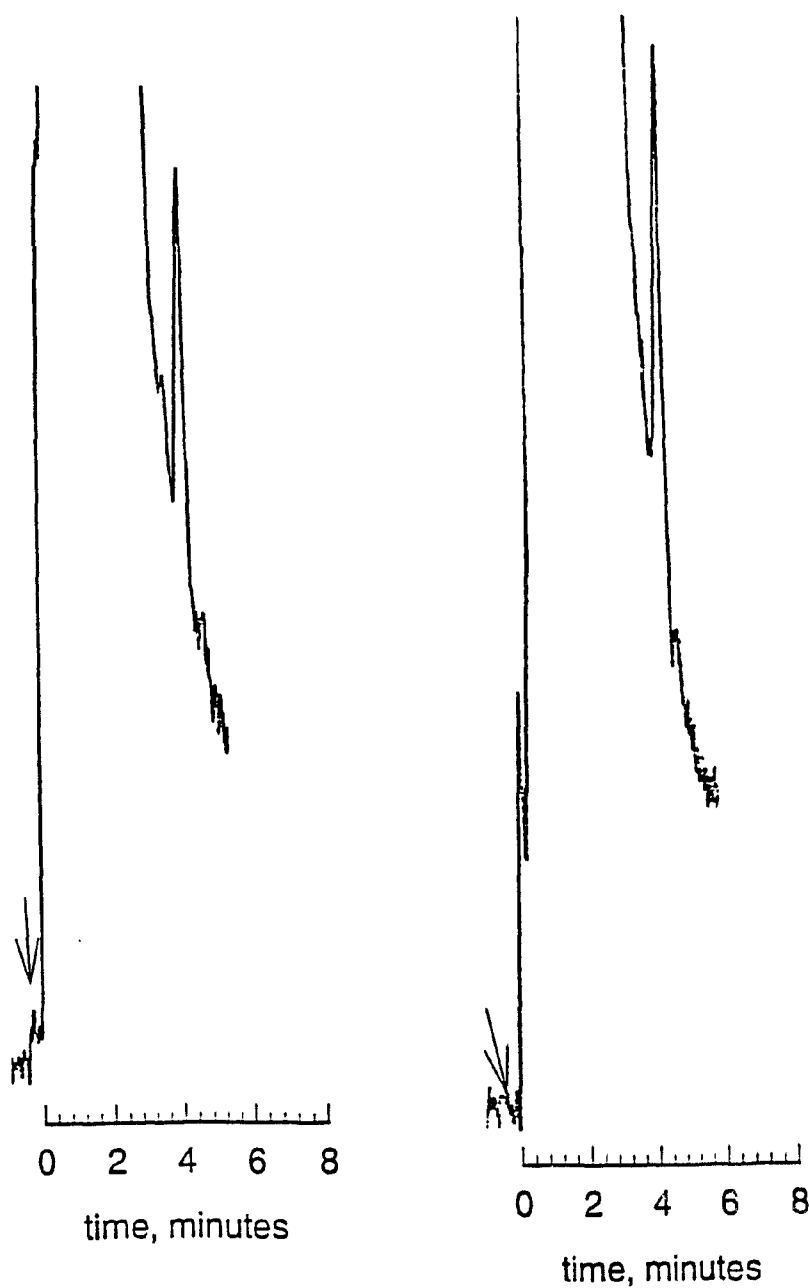
Figure 6.17 MDL peaks and values for tungsten hexacarbonyl: R-1104, -560 V; 455 nm (LP); H 2 14 mL/min; N 2 28 mL/min; column 60 °C; RC time constant 1 second.
