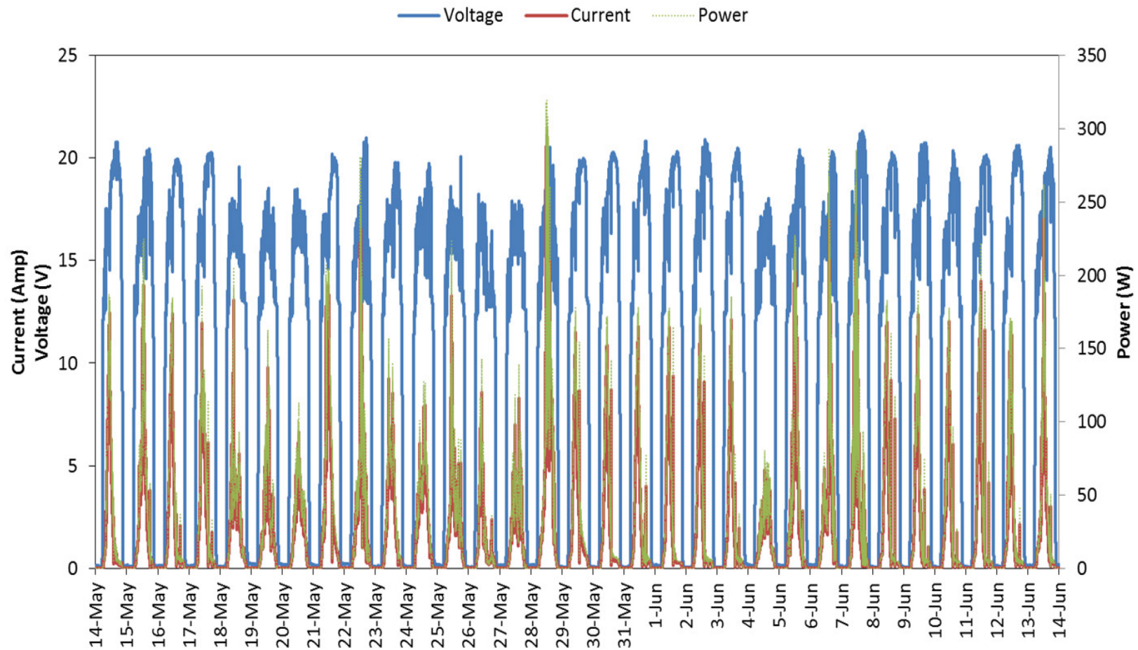
Figure 55: PV output voltage, current and power
