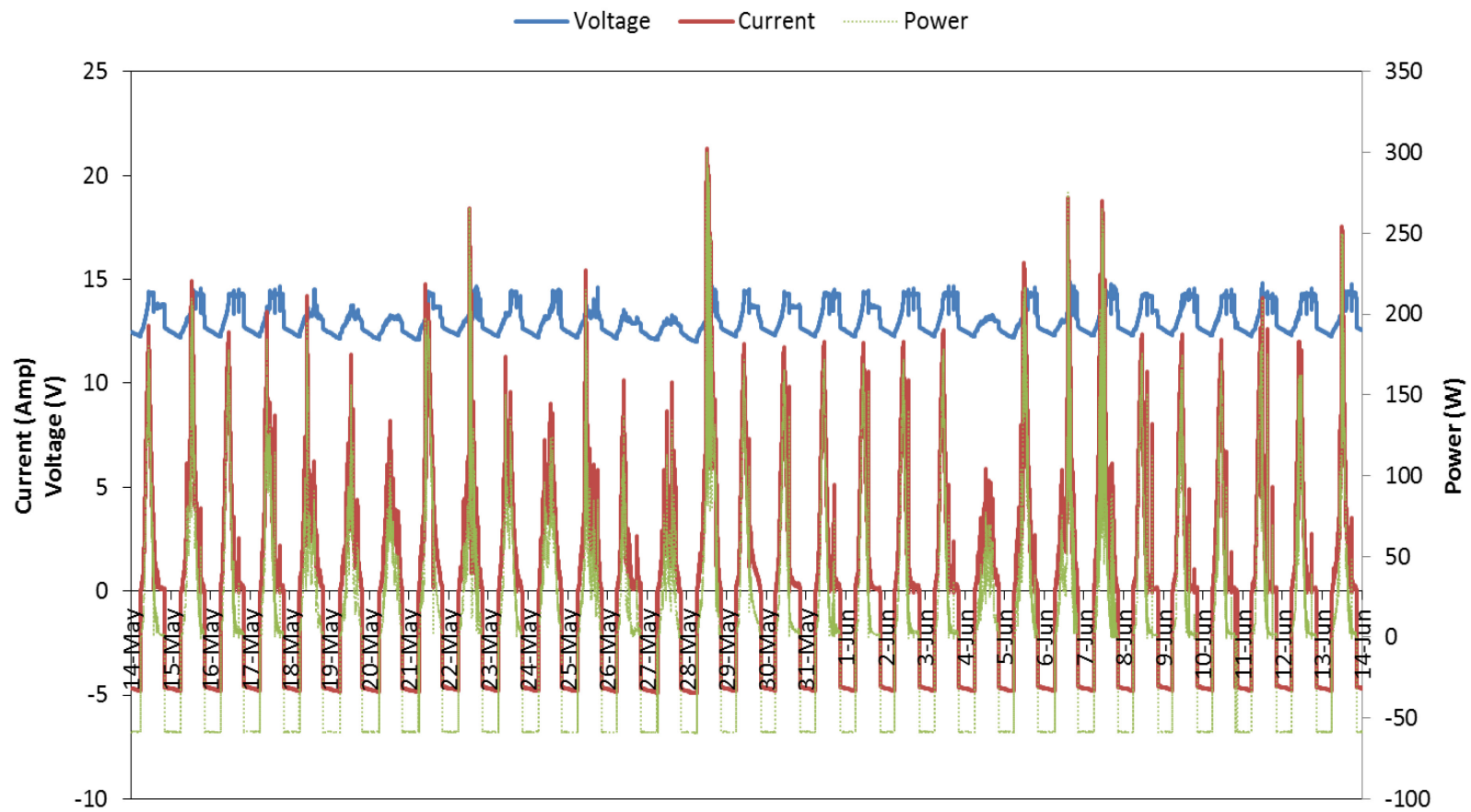
Figure 58: Battery voltage, current and power profile
