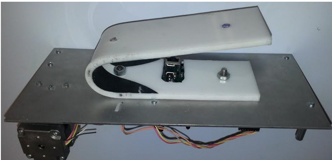
Figure 11: Photo of custom bracket mounted on scan head
