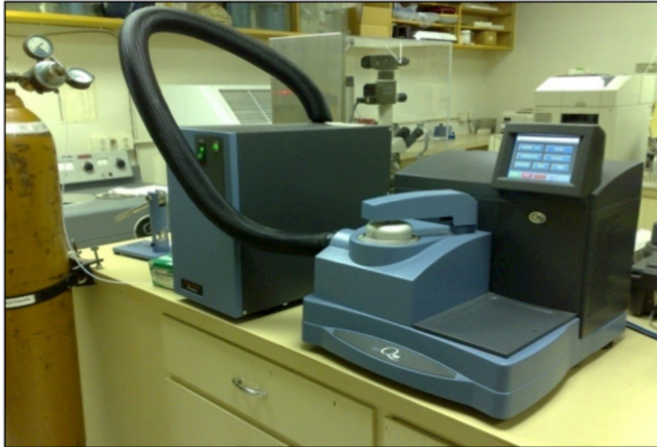
Figure 3- 3. TA Instruments heat flux DSC Q100 equipped with modulated® DSC connected to a refrigerated cooling system, RCS (Al-Qatami, 2011)
