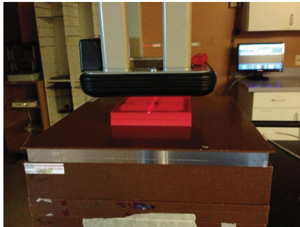
Figure 3.10 Dosimetric verification of bolus material. PLA slabs replaced the superficial 1 cm of solid water.
