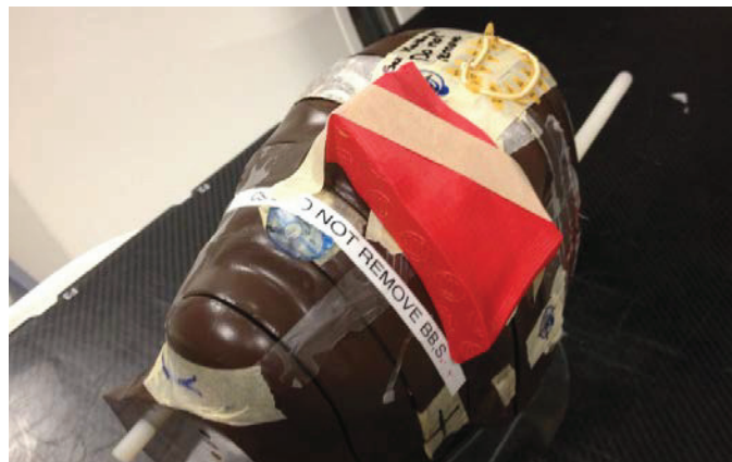
Figure 4.9 Picture of head phantom with bolus added on the surface
