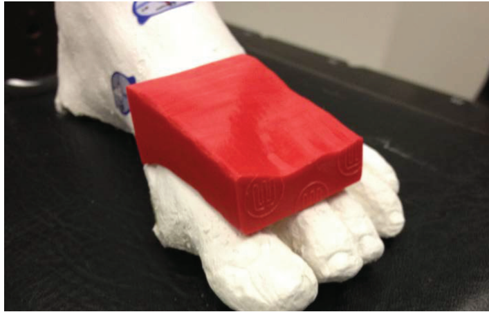
Figure 4.5 Picture of foot phantom with bolus added on the surface
