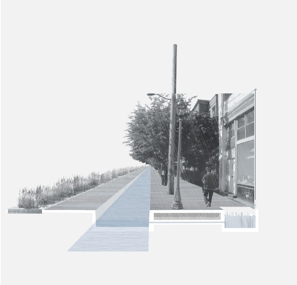
Intake to waterway: sectional study with visible bioswale strip and reed bed.
