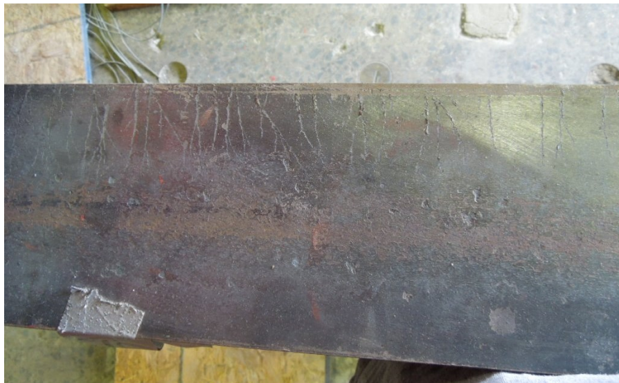
Figure 4.11 Yielding of specimen C1-1 beam 2 compression flange.
