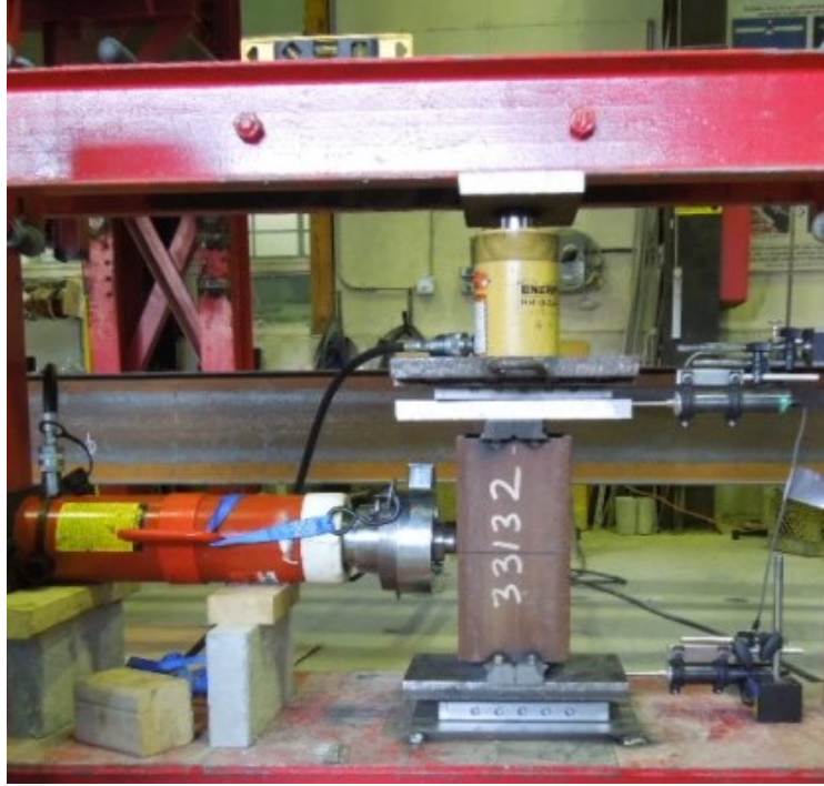
Figure 5.8 Specimen C1-1 roller friction experiment.
