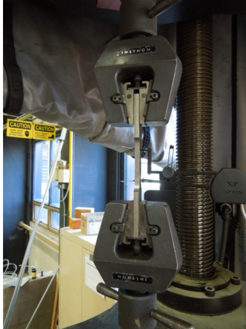
Figure 3.23 Tension coupon test setup.
