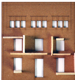
Initial studies of lighting and framing the openings, as viewed from the back of the facade
