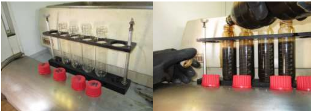
Figure 4.14 Filling the prescription bottles with fresh crude oil.
