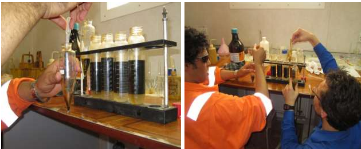
Figure 4.32 Sub-sampling the treated bottles (10, and 12.5 ppm. of 2137-T).
