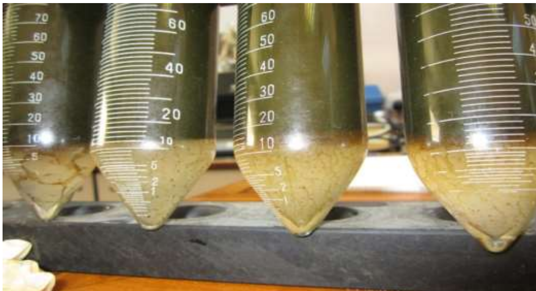
Figure 4.25 3-prescription bottles treated with 15 ppm dosage of Blend-X, after 7 minutes (blank sample-left).
