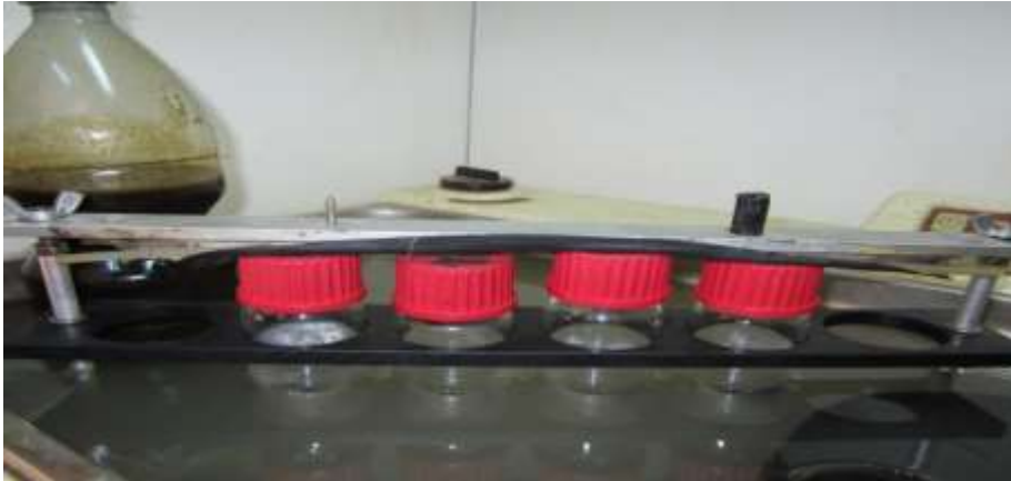
Figure 4.11 Heating up empty bottle-test kit.
