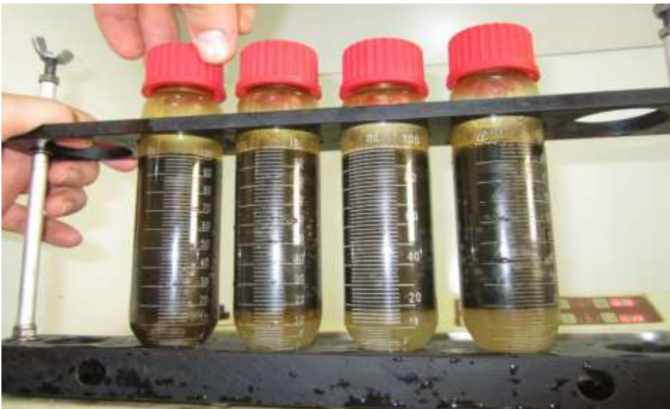
Figure 4.29 The heated bottles out of the water bath for shaking.
