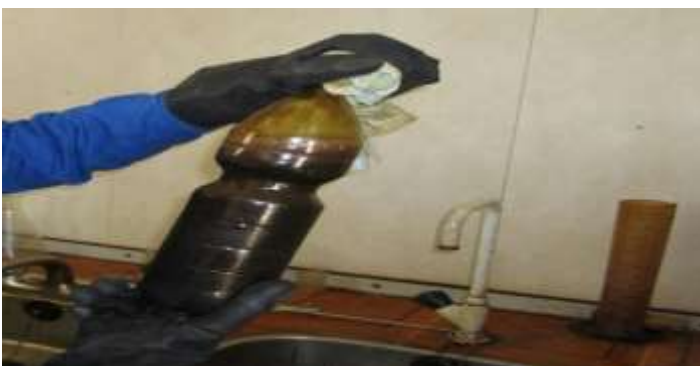
Figure 4.13 Freeing the gases out of crude oil sample.
