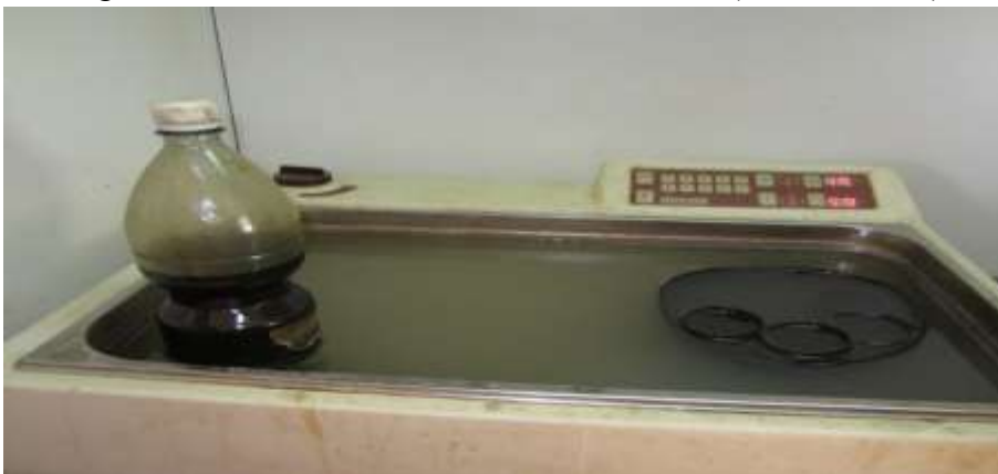
Figure 4.10 Heating up the fresh crude oil samples.
