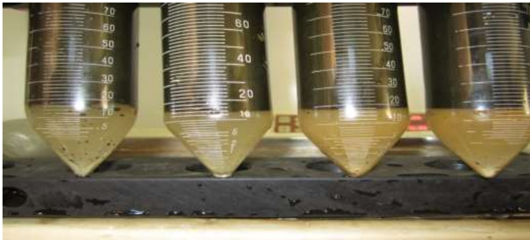
Figure 4.24 3-prescription bottles treated with 10 ppm of Blend-X after 7 minutes (blank sample-left).
