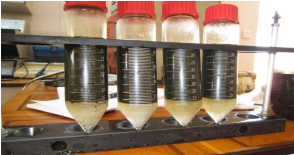
Figure 4.21 The 3- prescription bottles treated with 10 ppm dosage of 2137-T, after 7 minutes (blank sample-left).
