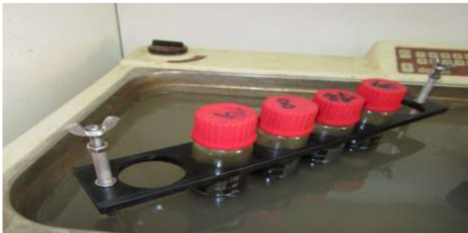
Figure 4.30 After shaking, the bottles again in the water bath for heating.
