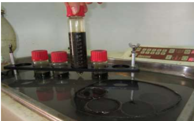
Figure 4.15 Heating up the 4 prescription bottles using the water bath.
