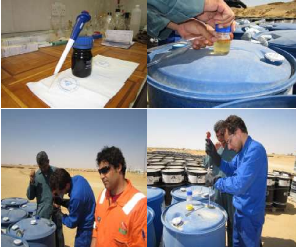
Figure 4.6 Preparing the demulsifiers samples.
