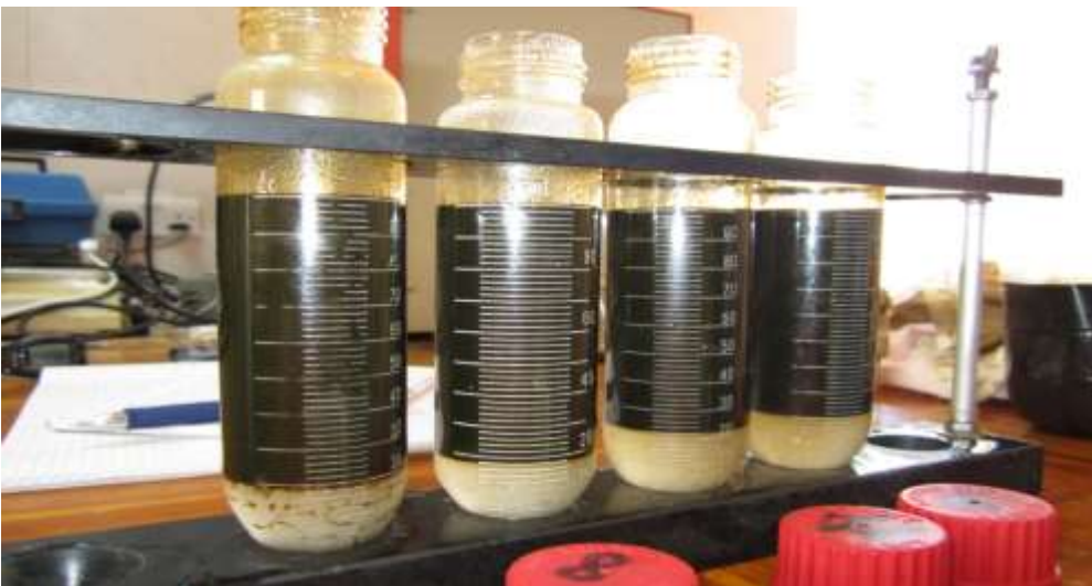
Figure 4.22 The 3-prescription bottles treated with 15 ppm dosage of 2137-T, after 7 minutes (blank sample-left).
