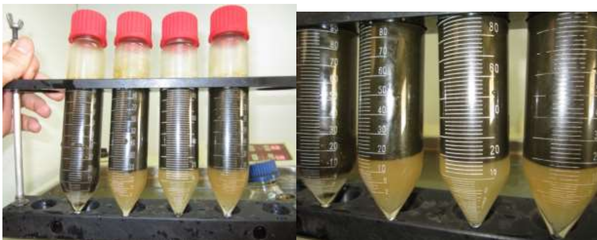
Figure 4.31 Adding 10, 12.5 and 15 ppm dosages of 2137-T to fresh crude oil samples (blank sample-left).
