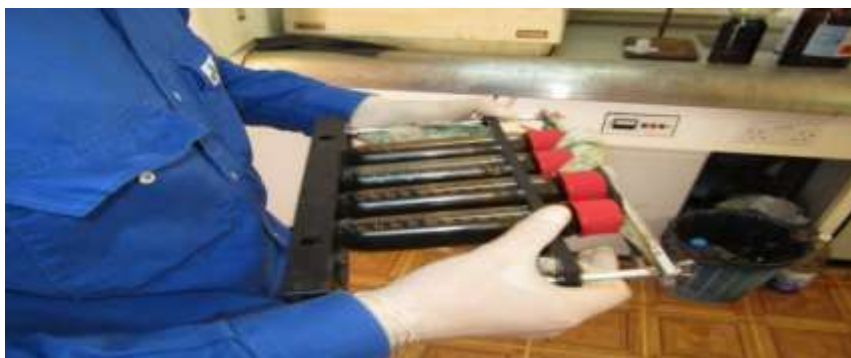
Figure 4.18 Shaking the treated prescription bottles.
