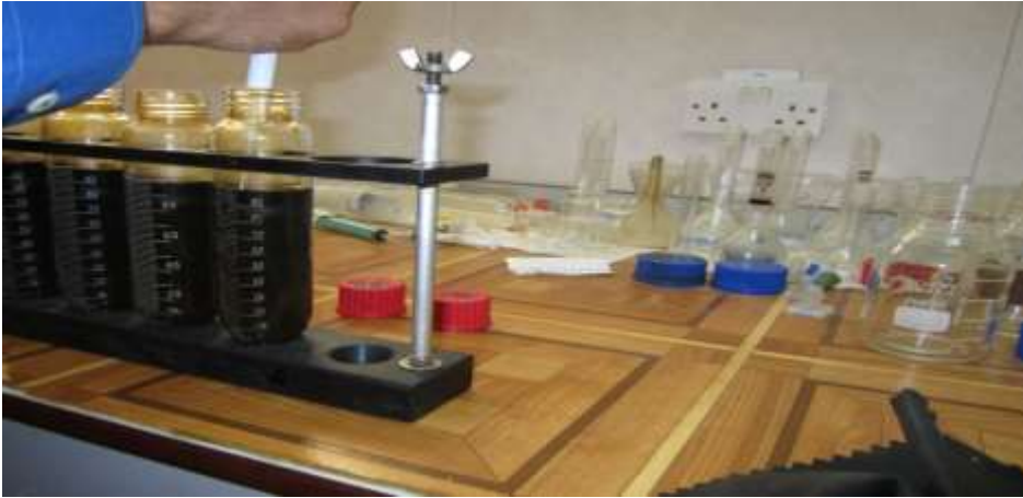
Figure 4.27 Adding different dosages of 2137-T to fresh crude oil samples (blank sample-left).
