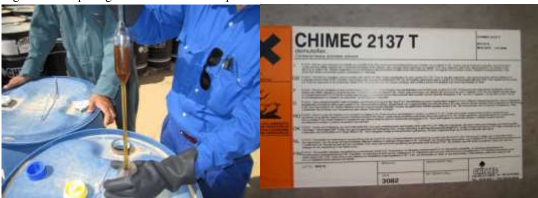
Figure 4.7 Preparing 2137-T demulsifier sample.
