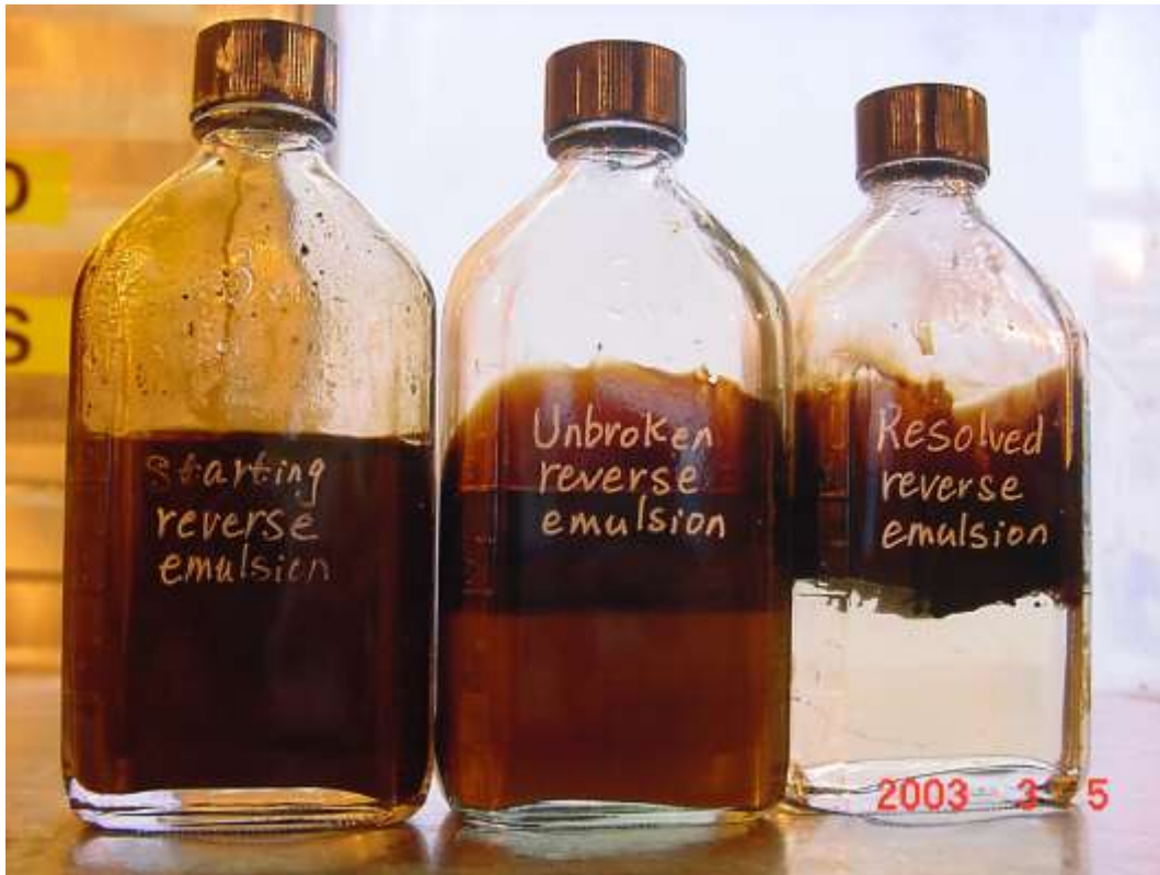
Figure 2.4 The effects of injecting not injecting any demulsifier (left), wrong demulsifier (middle), and injecting the right demulsifier (right) (Institut français du pétrole, IFP Training, 2009).
