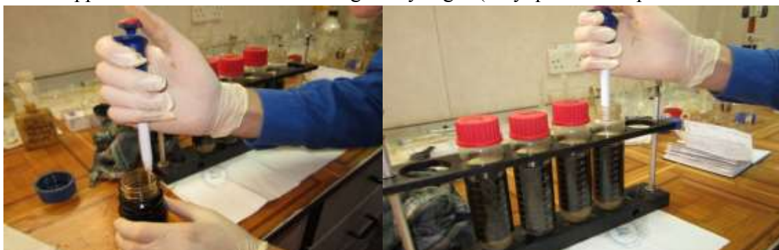
Figure 4.17 Adding 10 ppm dosage of 2137-T to 3 prescription bottles.
