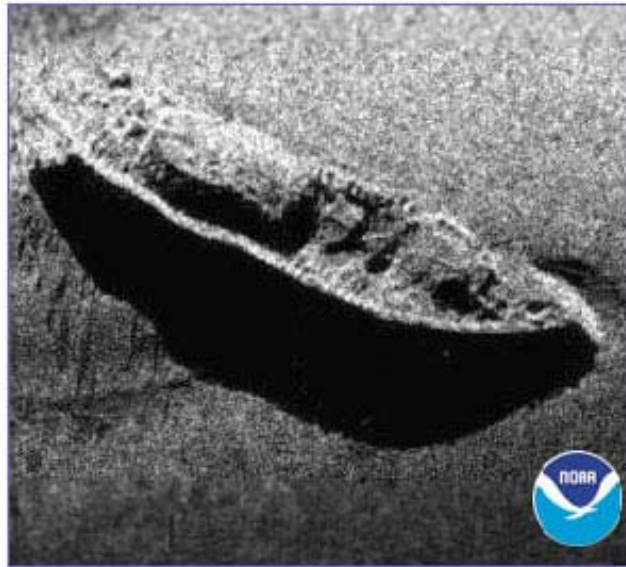
Figure 5.2: Side scan sonar image of the wreck. Image taken from [1]
