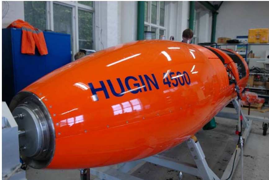
Figure 1.1: Hugin 4500 autonomous underwater vehicles. When submerged, the vehicle uses dead reckoning, incorporating Doppler velocity log and compass input to maintain an estimate on current positioning.
