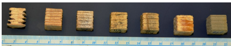
Figure 3.5: Wood blocks that have been cleaned after incubation. The treatments from left to right are as follows: Control, 100D, Dcunap, 30/70BDWS, 50/50BDWS, 100BDWS, and CCA.
