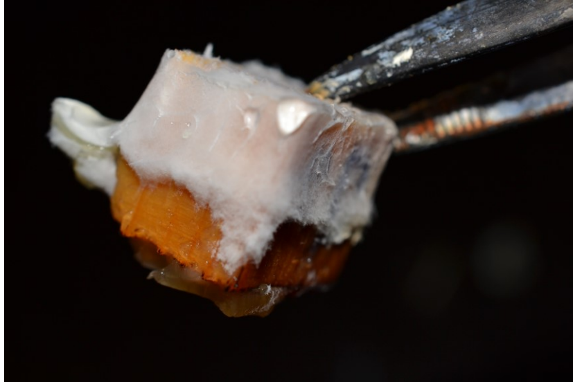
Figure 4.1 : A Douglas fir sapwood block treated with 100BDWS showing the encapsulating layer of fungal mycelia of P. placenta .
