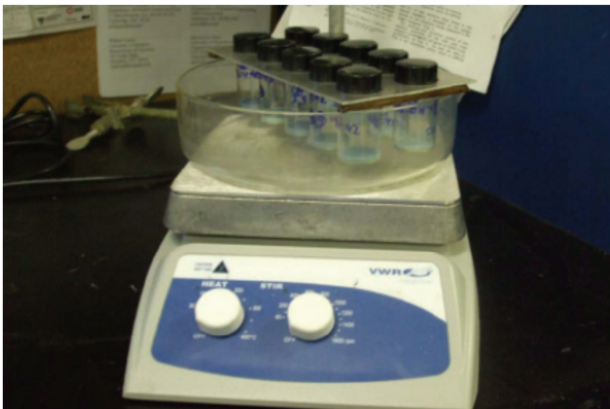
Figure 3.4. The experimental setup used during heat/cool cycling experiments. The heating rate was controlled by the hot plate and the cooling rate was controlled by the addition of ice to the water bath. The temperature was recorded by a mercury thermometer held in the water bath and the samples were held in the bath by a sheet of aluminium.
