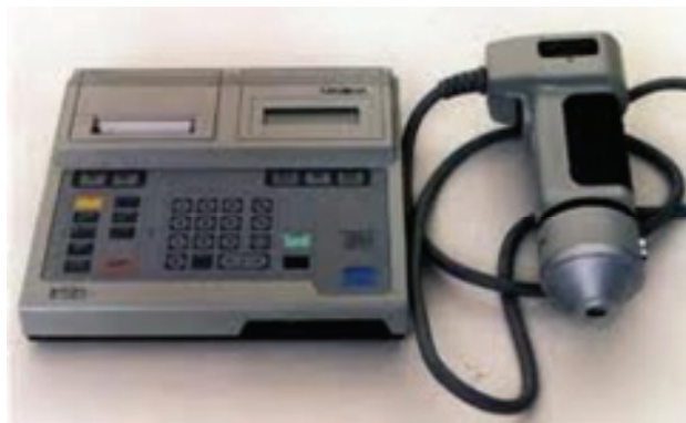
Figure 3.11. The Konica Minolta Chroma Meter CR300 used to analyze the colour of printed images.
