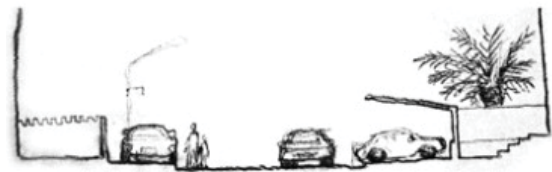
Section through of a recent neighborhood street in Ahmedi, Kuwait, showing the lack of space for a side walk and the car shading structure.
