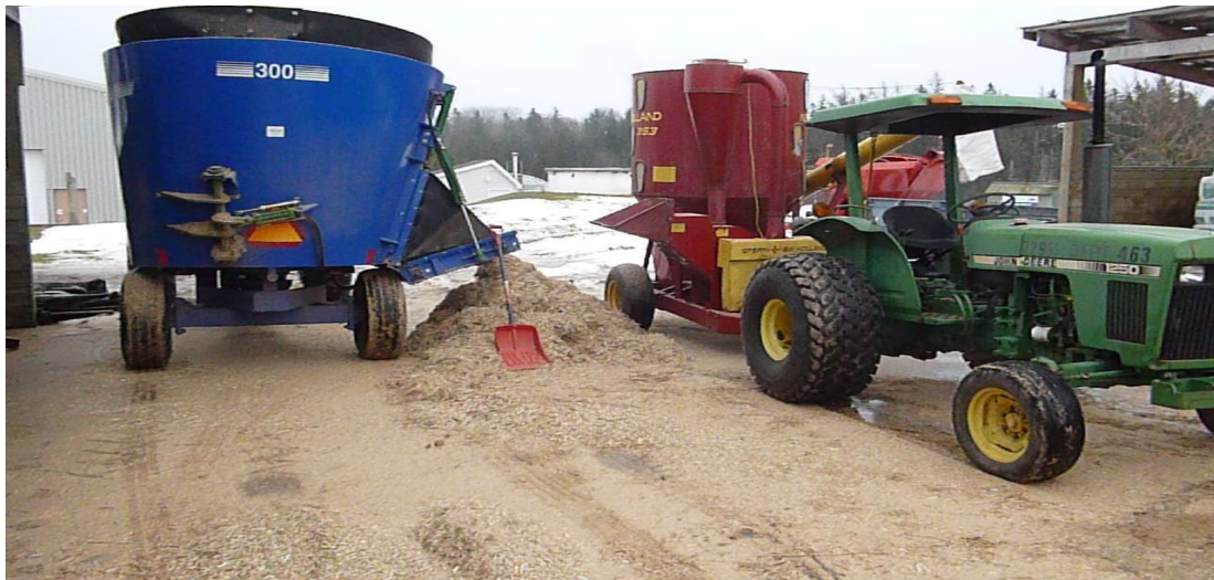
Figure 1. Feedstock preprocessed in a Supreme Enviro pull type TMR mixer.
