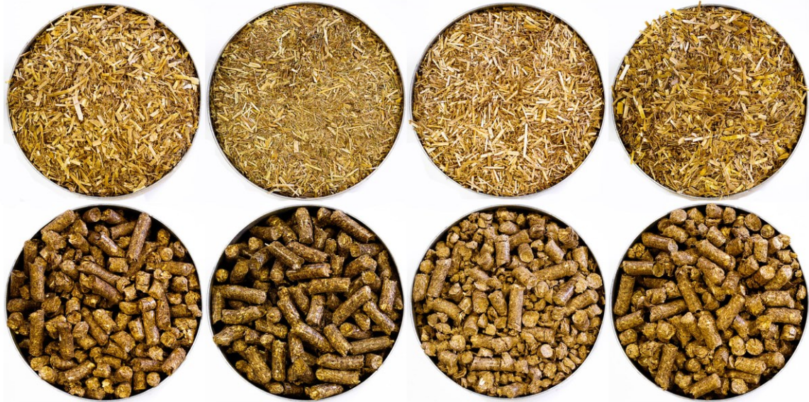
Figure 4. Pellets (bottom row) and hammer milled feedstock (bottom row) from which pellets were produced. (Left to right) Barley straw, Reed canary grass, Switch Grass and Wheat straw.
