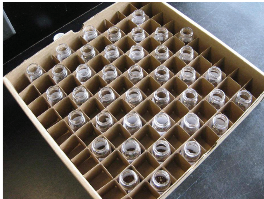
Figure 3.1 Experimental set up of performance test showing microcosms (test vials) filled with field or OECD soil, maize and/or yeast, arranged in randomized order.
