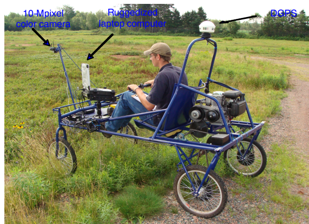
Figure 1. Configuration of automated yield monitoring system mounted on farm motorized vehicle.
