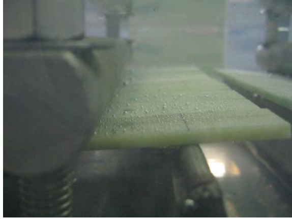
Figure 5.3 Specimens under external load immersed in acid
