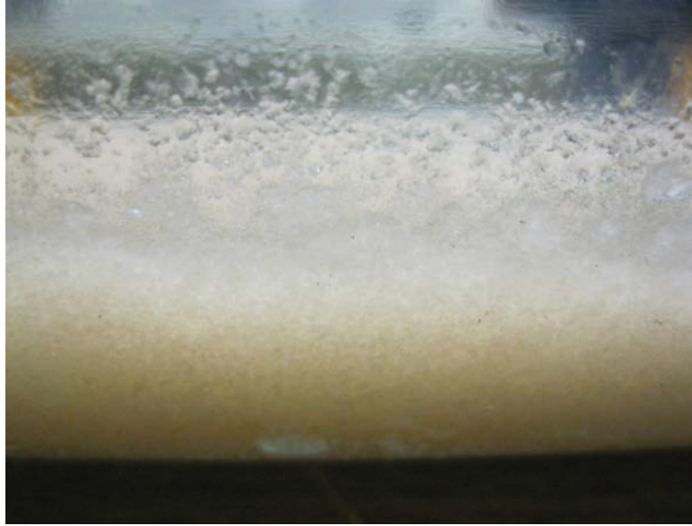
Figure 5.8 White precipitation as a result of chemical reactions between the fibers and sulphuric acid
