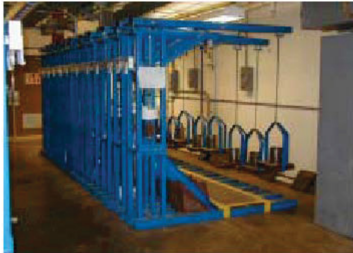
Figure 2.15 Tensile loading frames used for acid corrosion resistant experiments [63]
