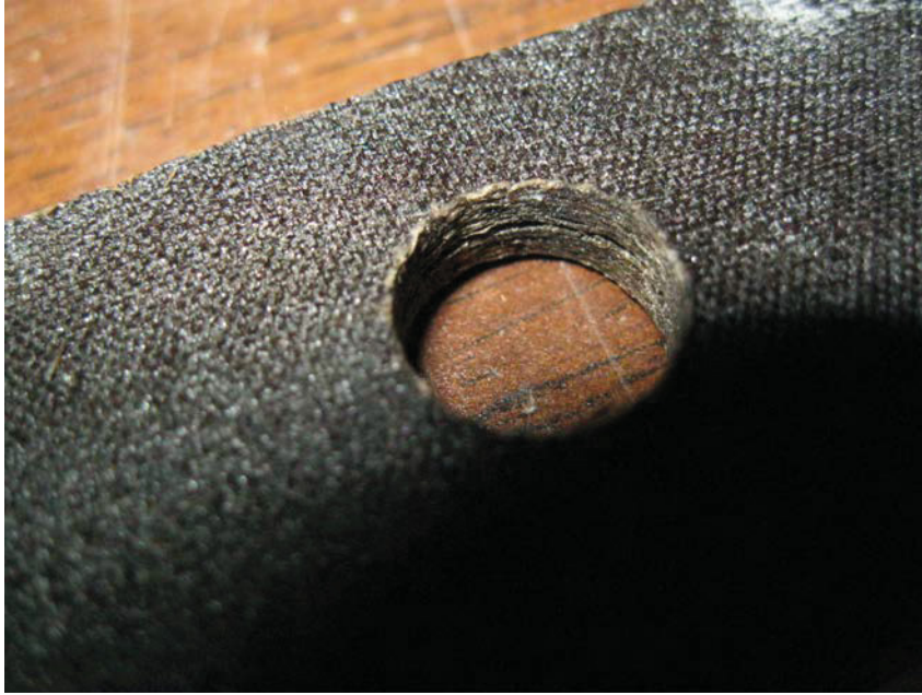
Figure 5.15 Typical delamination seen in the specimens due to the chemical degradation of the resin and fibers
