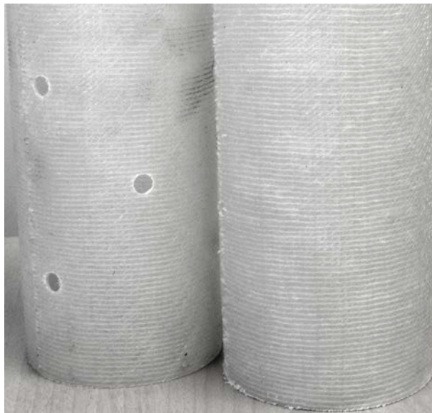
Figure 7.1 Typical perforated and non-perforated pipe specimens
