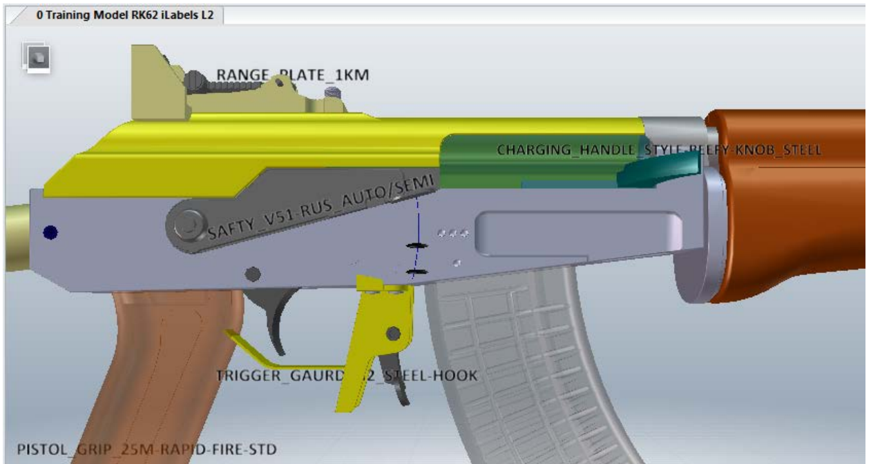
Figure 1: Training 3D model annotated with internal style textual annotations. The training model of RK-62 rifle was used to provide training on how to operate the 3D software used in the study and to make the participants familiar with the study setup and internal annotation style.
