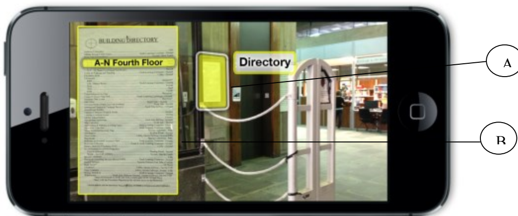
Figure 34: Highlighting the directory. View was captured through camera, it will automatically highlight important signage (A). User can see more detailed information by clicking on it (B)
