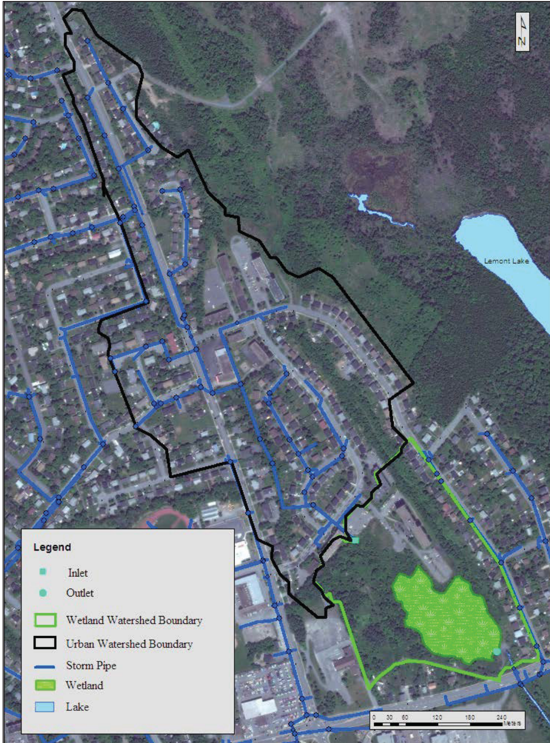
Figure 3-2 Watershed boundary detail with stormwater infrastructure
