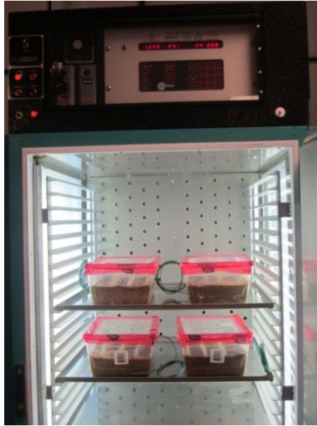
Figure 12: Experimental set-up inside the Germination Chamber with 4 replicates.
