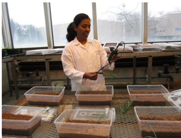
Figure 2: Monitoring soil moisture potentials using soil moisture sensor and sensor reader
