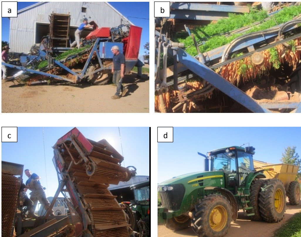
Figure 32: Machine operated carrot harvesting, a- carrot harvester with harvested carrots, b- carrots with top parts of the plant, c- conveyor belt to send carrots from the harvester to root collecting tractor, d- tractor to collect roots
