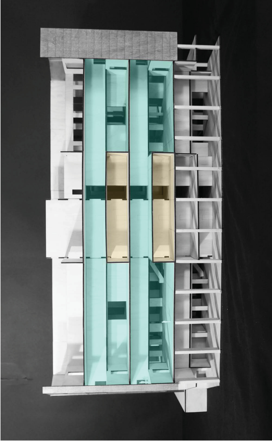
Highlighted model section showing the interweaving of large event and gallery spaces through floors (green) and smaller cellular spaces (yellow)
